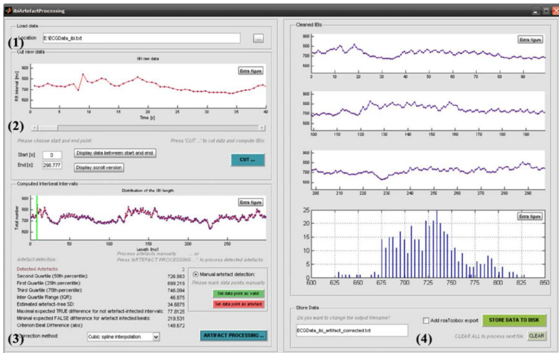
Figure 3: The graphical user interface of the sub program ibiArtifactProcessing. (1) load data, (2) raw data plot on a scrollable axis and the possibility to cut data manually, (3) data plot with detected artifacts and the possibility of manual intervention, (4) data plot showing the corrected IBIs and the histogram, (5) data storage
