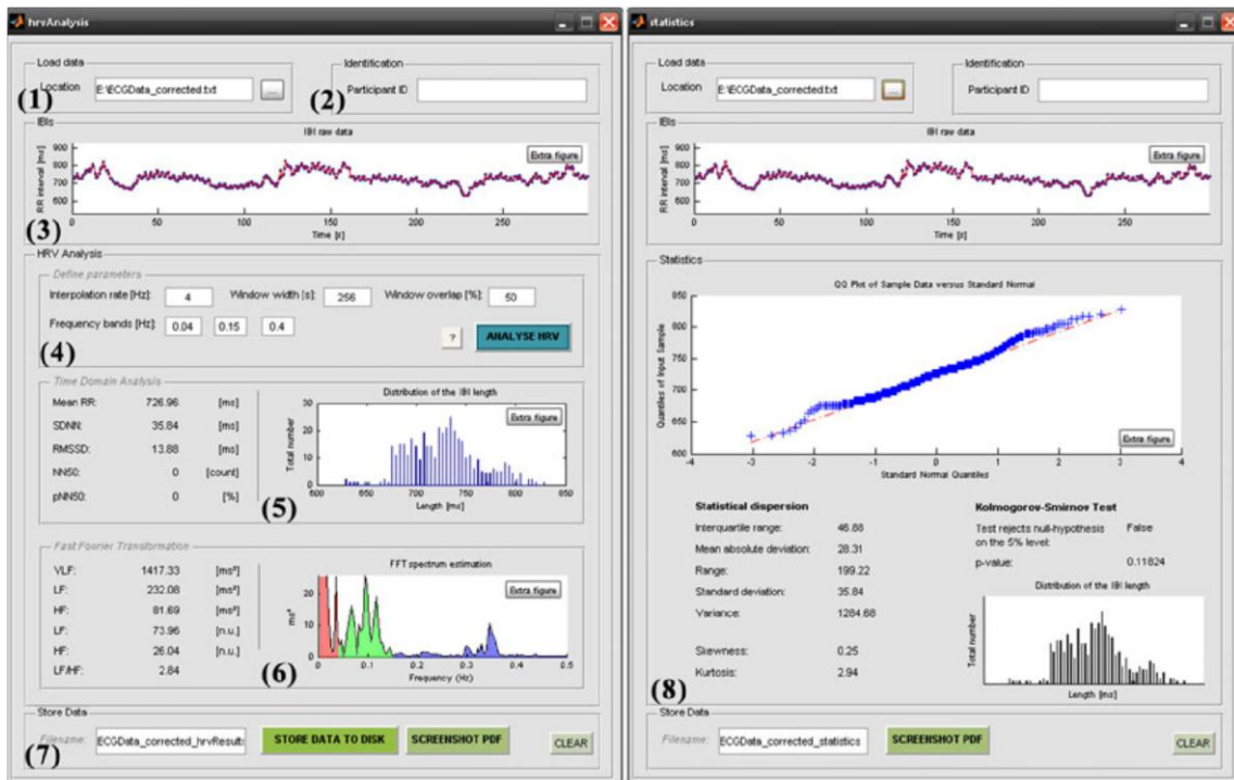
Figure 4: The graphical user interface of hrvAnalysis and descriptiveStatistics. (1) load data, (2) insert participant ID (optional), (3) raw data plot, (4) settings for HRV computation, (5) time domain analysis, (6) frequency domain analysis, (7) store data, (8) distribution statistics
